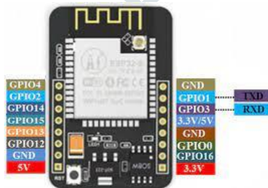
Figure 1. ESP-32 CAM Module
