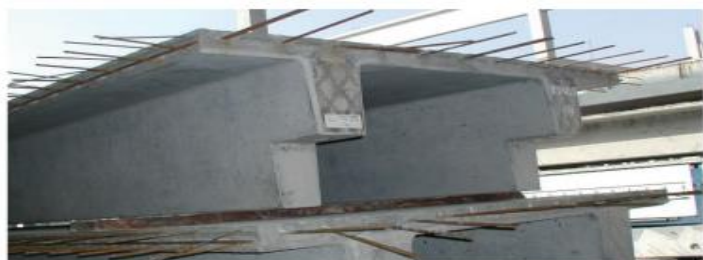
Fig1.1: Connection detail of post-tensioned precast specimen
