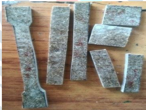
Fig. 8 Test specimen as per mentioned ASTM dimensions
