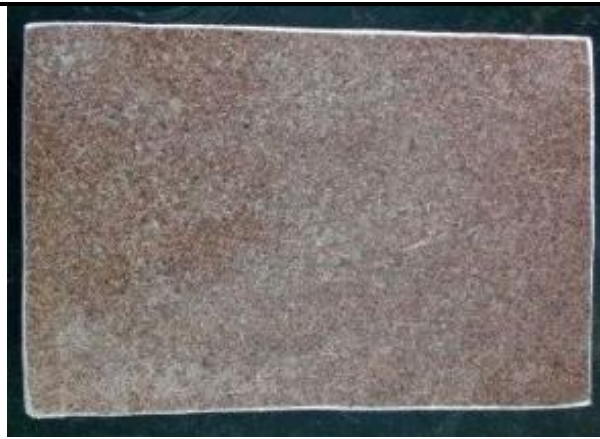
Fig. 6 Final edge grinded composite plate after curing
