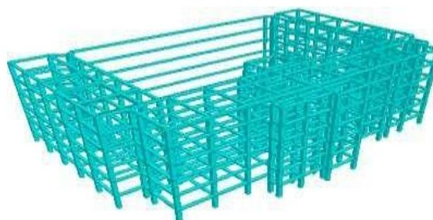
Figure 3: Stadd Pro plan of Without Expansion Joint
