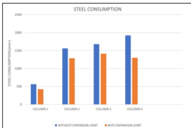
Figure 9: Comparison of Steel Consumption in Column
