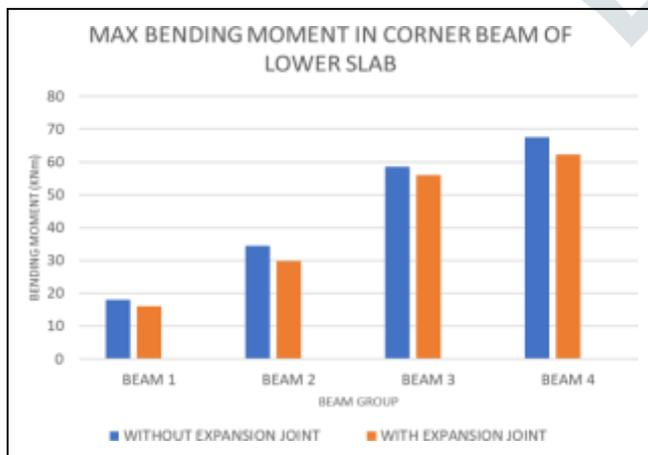
Figure 5: Comparison of Maximum Bending Moment in Corner Beam of Lower Slab
