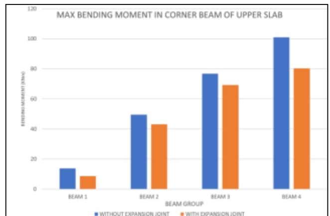
Figure 7: Comparison of Maximum Bending Moment in Corner Beam of Upper Slab
