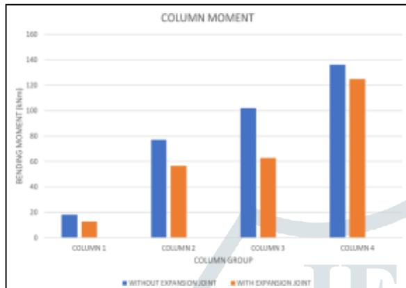
Figure 8: Comparison Of Maximum Moment In Column
