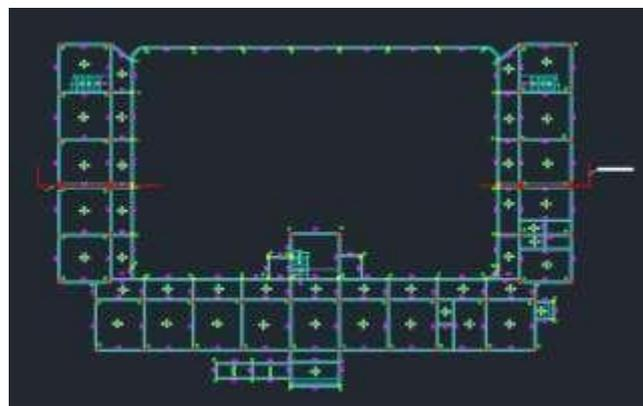
Figure 2: AutoCAD plan of Structure is considered with expansion joint.
