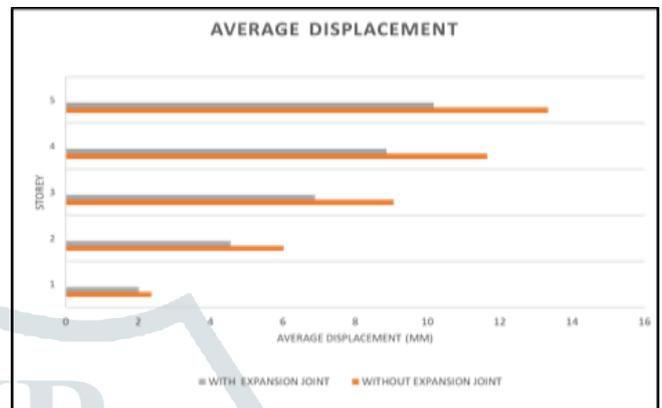
Figure 10: Comparison of Average Displacement in Column
