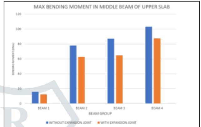
Figure 6: Comparison Of Maximum Bending Moment In Middle Beam Of Upper Slab
