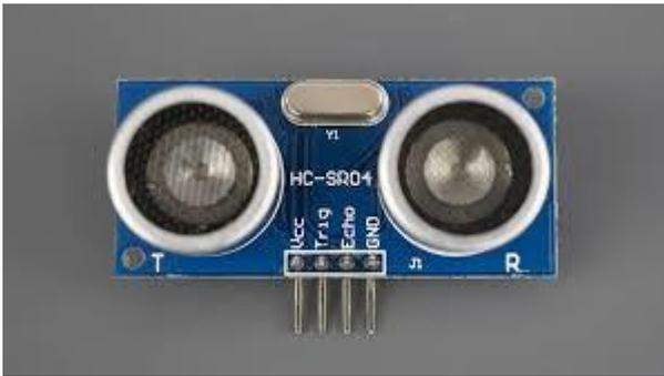
**Fig. Ultrasonic Sensor**
