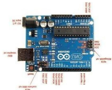
Fig. Image of an Arduino UN
