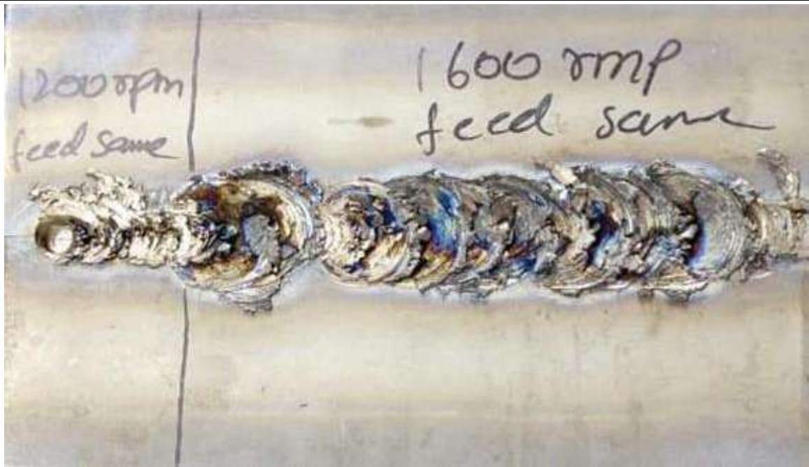
Fig1.3: FSW on Titanium Sheet
