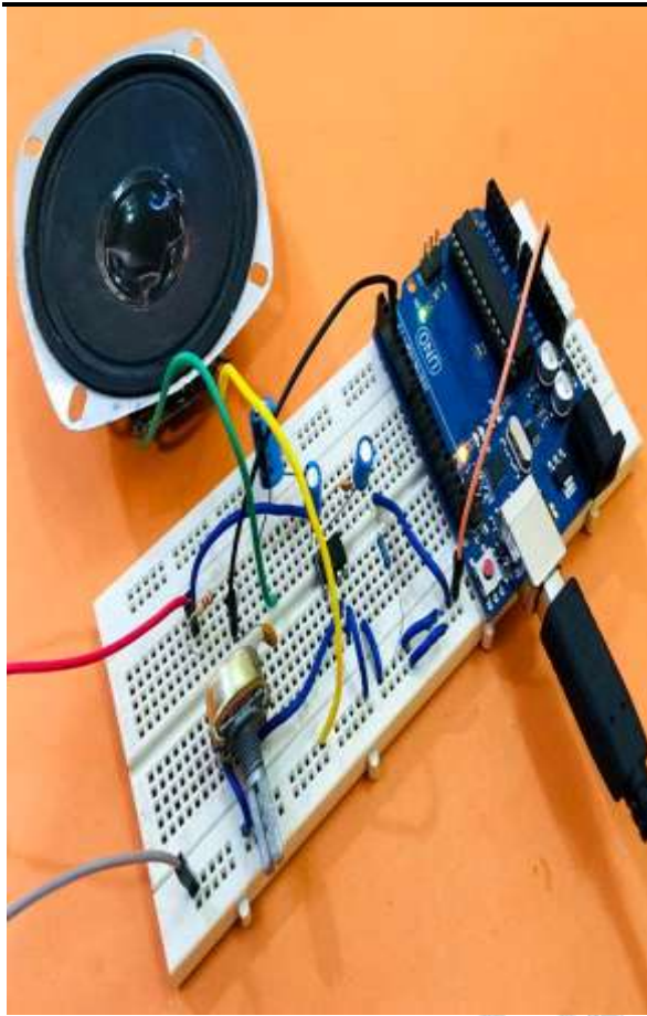
Figure 2 : Arduino Based Text To Speech Converter
