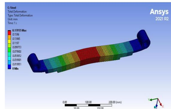
Deformation results of Mild Steel Leaf Spring
