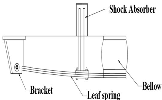
**Schematic diagram of leaf spring assembly**
