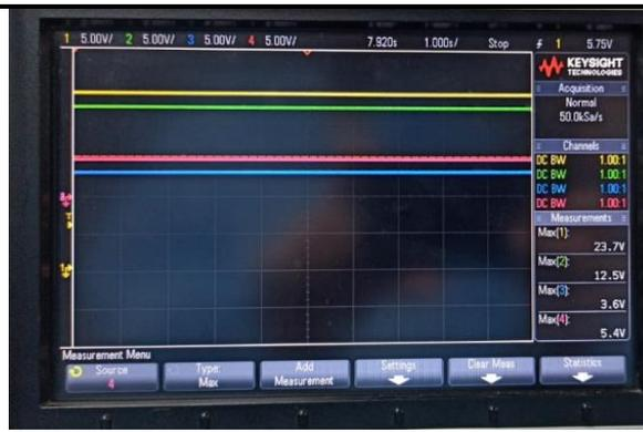
Fig4.5 Multiple outputs of forward converter
