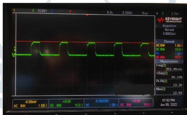
The waveform of drain to source voltage waveform of MOSFET is shown in the Fig4.4. stress on the switch is high without snubber circuit.
