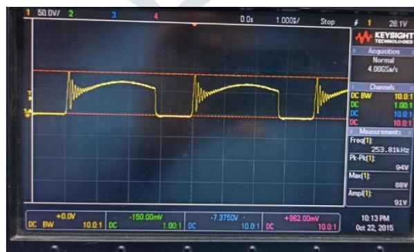
The secondary side of the forward transformer are designed to get output voltage of 24V from synchronous buck converter with input raw voltage of 36V and other raw voltages of 14V,6V and 4V further connected to LDO regulators to regulate these voltages to 12.7 V, 5.6V and 3.8V respectively is shown in Fig4.5
