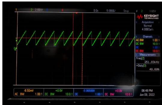
Fig4.2 Ramp voltage waveform
