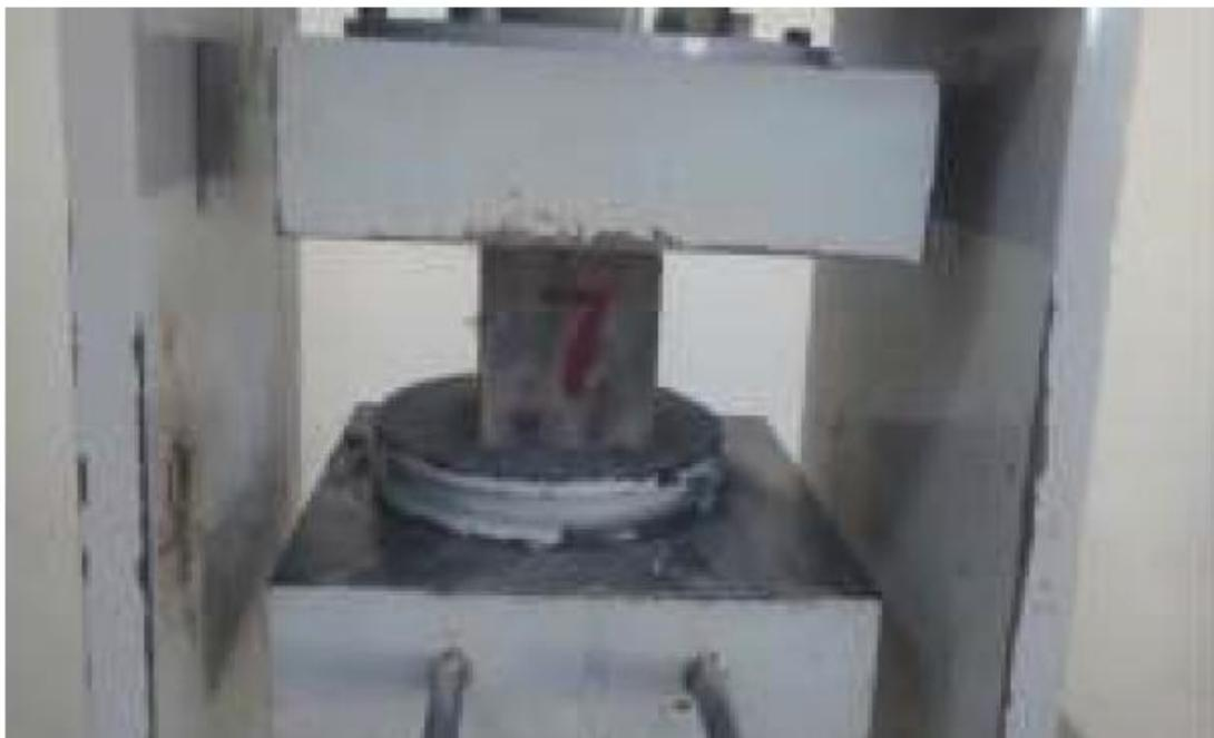
**Figure 3.3. Compression test on cube specimen**
