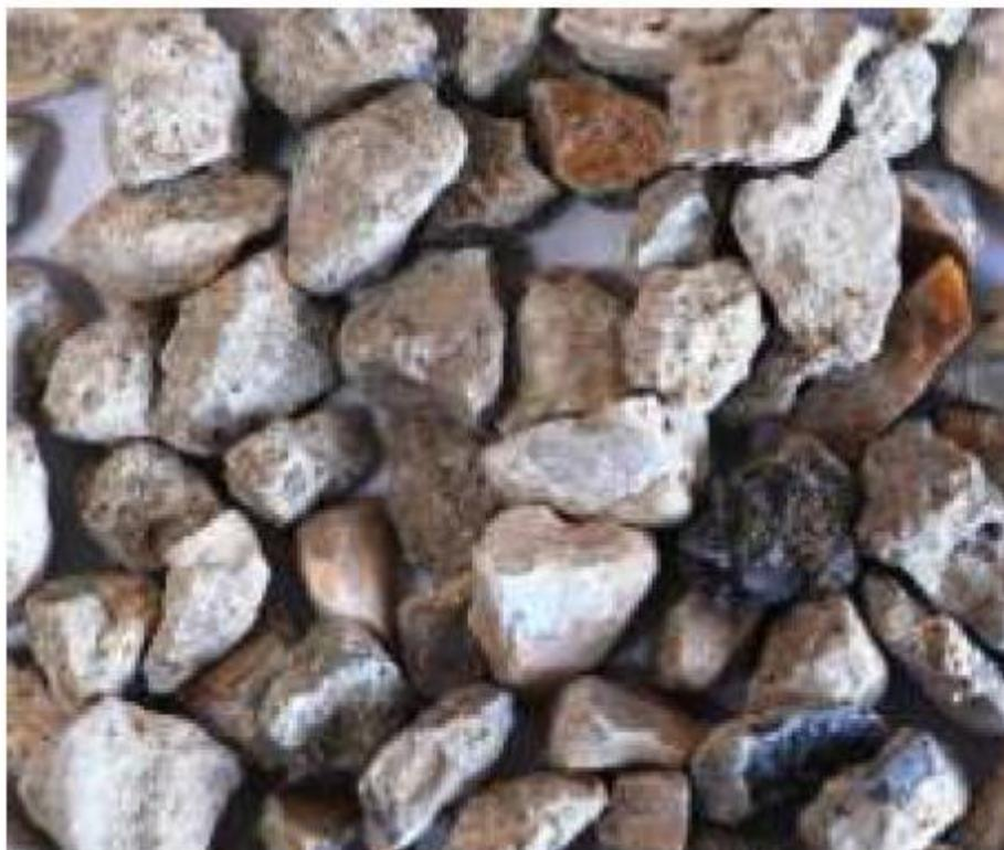
**Figure 3.2 Sample of RCA used in the study**
