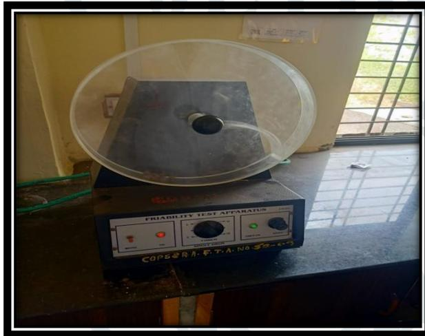
**Fig.2: Friability Test Apparatus.**
