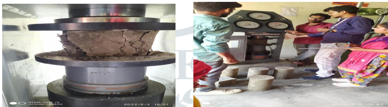
Figure 5.3 Testing compressive strength for cube in UTM
