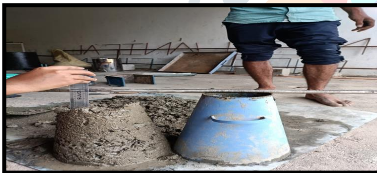
Figure 5.1 Slump cone test for concrete mix
