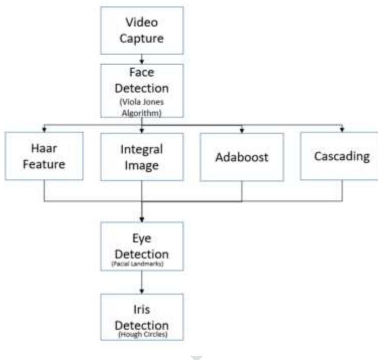
Fig 3: Block diagram for Iris Detection
