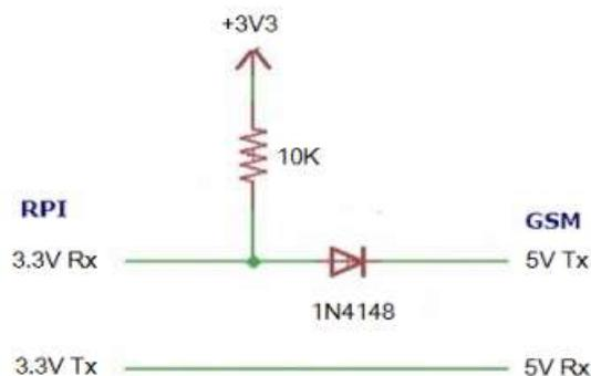
Fig 2: Level Shifter Circuit
