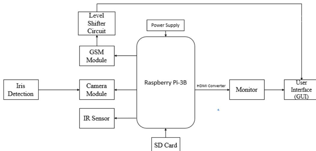
Fig 1:Hardware Block diagram
