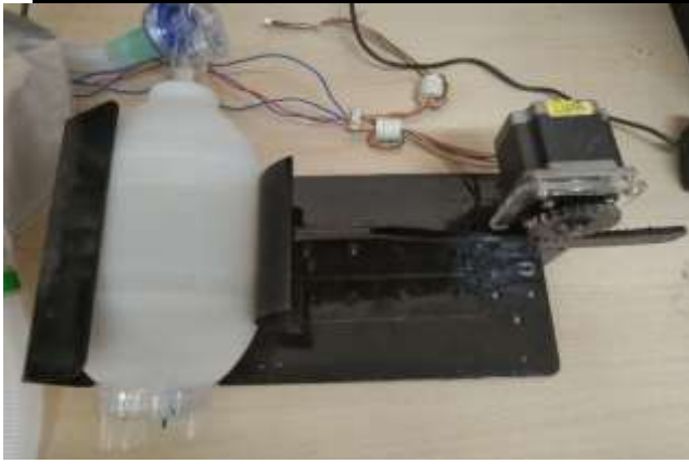
Figure 3: Top view of ventilator model
