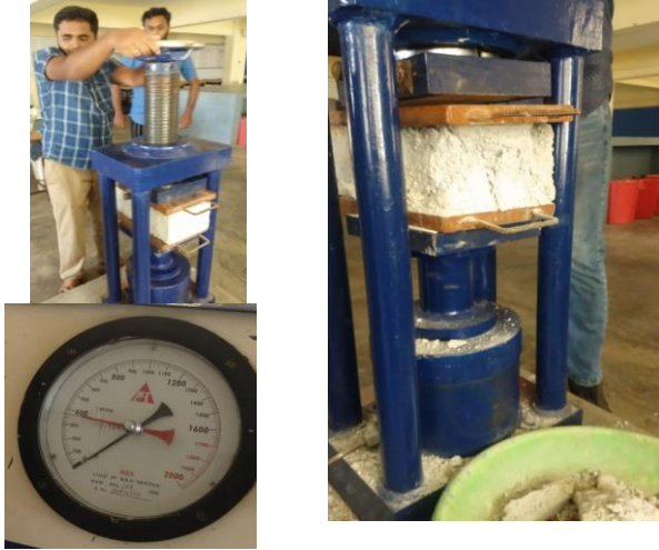
Figure 4: Conc. Block Lab Test
