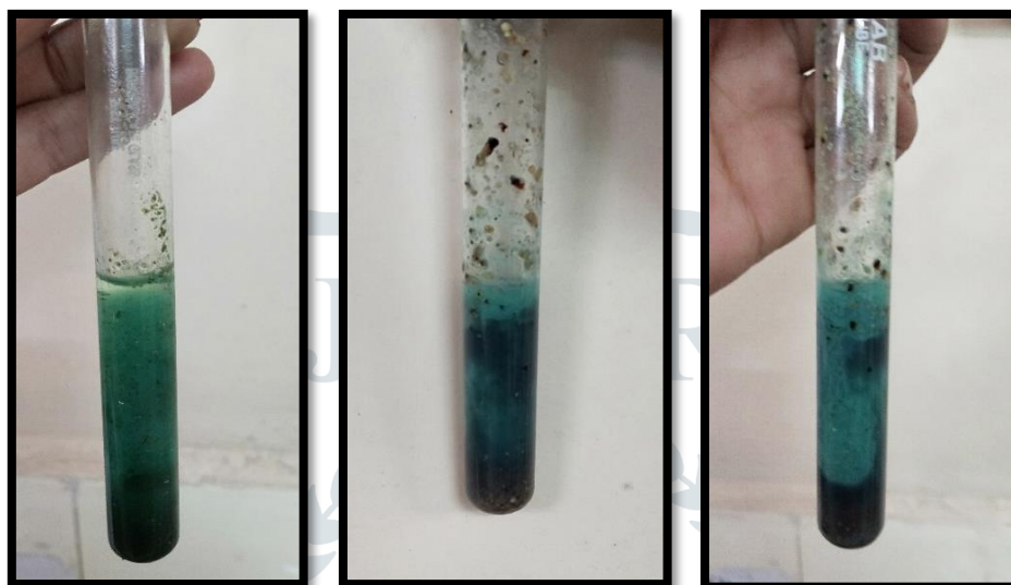
Fig: It indicate that the Gelatin test of Tannin produces blue color it means that the sample test for tannin is found positive.
