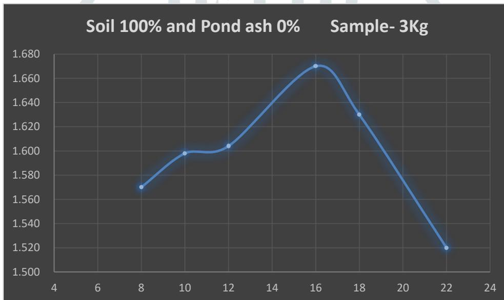
**Fig.3: Proctor test data**
