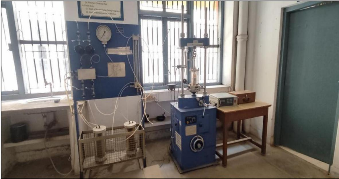
**Fig.4: Traixial testing machine**
