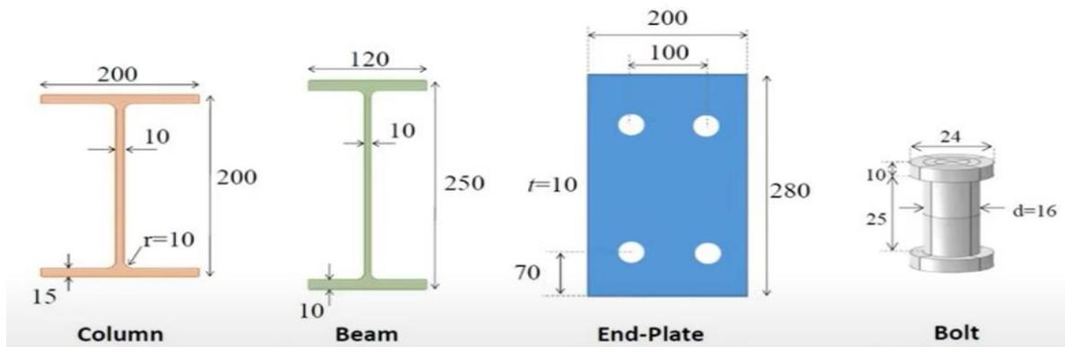
Fig.3 Dimensions of end plate steel beam-column connection
