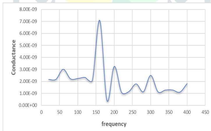
Fig. 5.a. Conductance vs frequency signature of healthy model.
