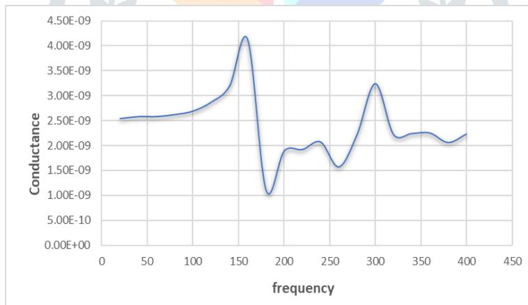
**Fig. 7.a.** Conductance vs frequency signature of retrofitted model.
