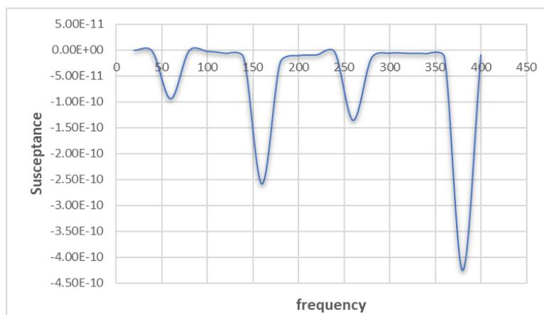
**Fig. 7.b.** Susceptance vs frequency signature of retrofitted model.
