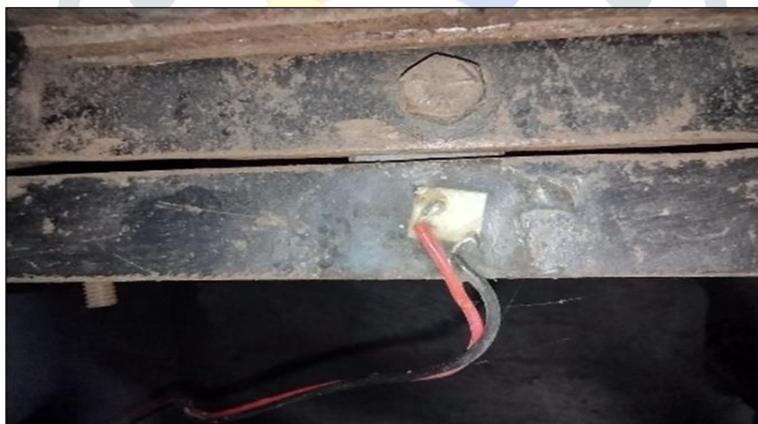
**Fig.1** Lead Zirconate Titanate (PZT) patch.
