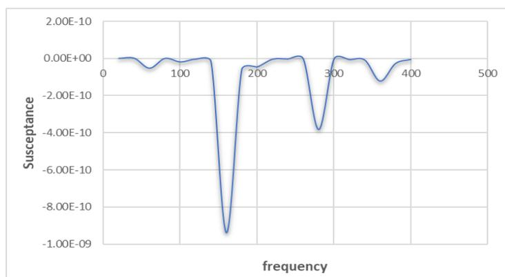
Fig. 5.b. Susceptance vs frequency signature of healthy model.
