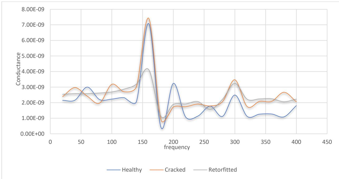
Fig. 8.a. Conductance vs frequency signature of all models.
