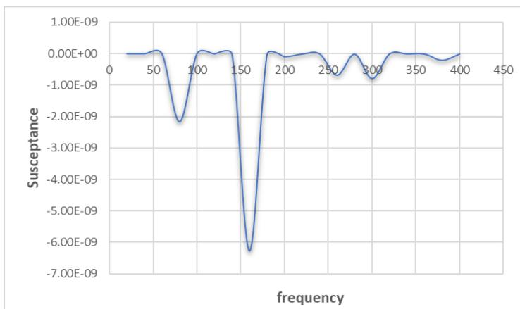
**Fig. 6.b.** Susceptance vs frequency signature of Cracked model.
