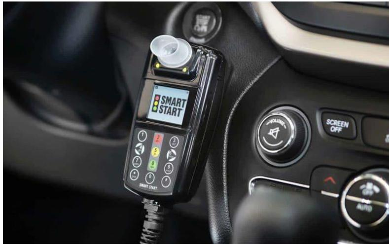
Fig 1: Ignition interlock device integrated in car (Source: Smart Start)
