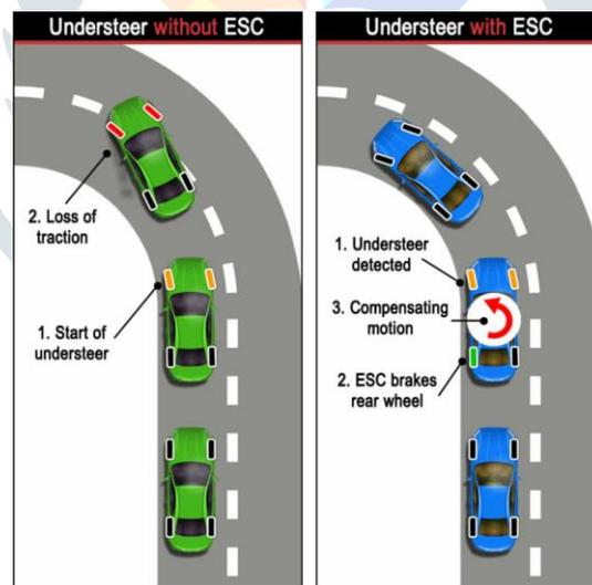
Fig 2: Electronics stability Control
