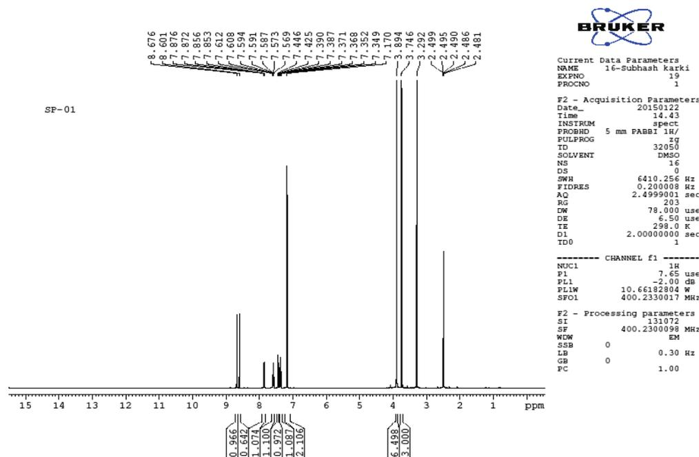
**Figure No.-04:**  $^1\text{H-NMR}$  Spectra of 3-(2-(3,4,5-trimethoxyphenyl)imidazo [2,1-*b*] [1,3,4] thiadiazol 6-yl)-2*H*-chromen-2-one. [CH69]
