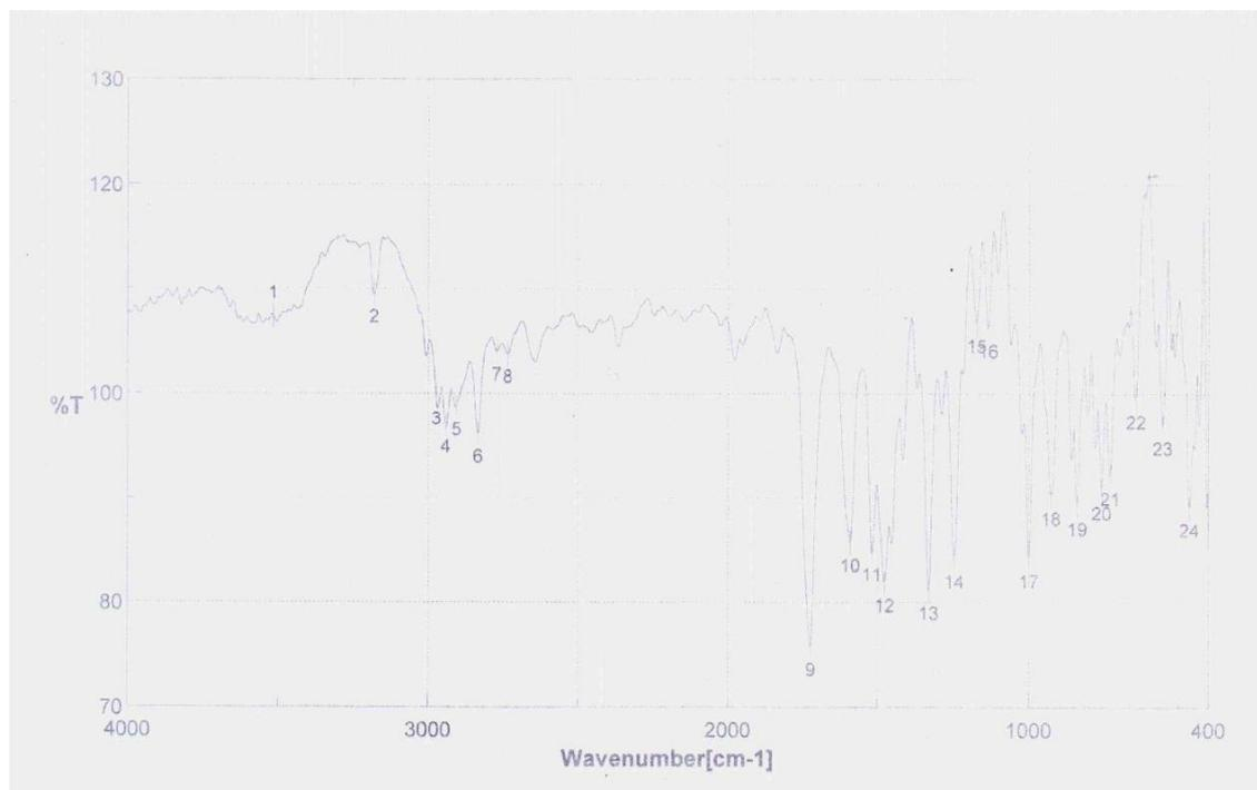
**Figure No.-03:** IR spectra of 3-(2-(3,4,5-trimethoxyphenyl)imidazo [2,1-*b*] [1,3,4] thiadiazol 6-yl)-2*H*-chromen-2-one.[CH69]
