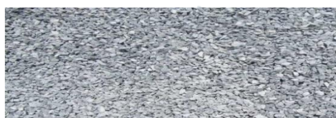
Fig. 3: 10 mm Size Coarse Aggregate
