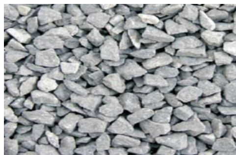
Fig. 2: 20 mm Size Coarse Aggregate
