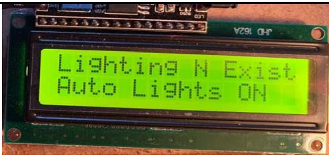
**Fig.11: LCD Shows that the Lights ON when NO Light Exist**
