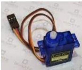
**Fig.9: Servo Motor**
