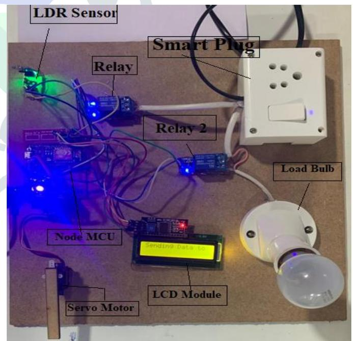
**Fig.10: Designed hardware kit for Smart Lighting, Smart Plug, Smart Gate System**
