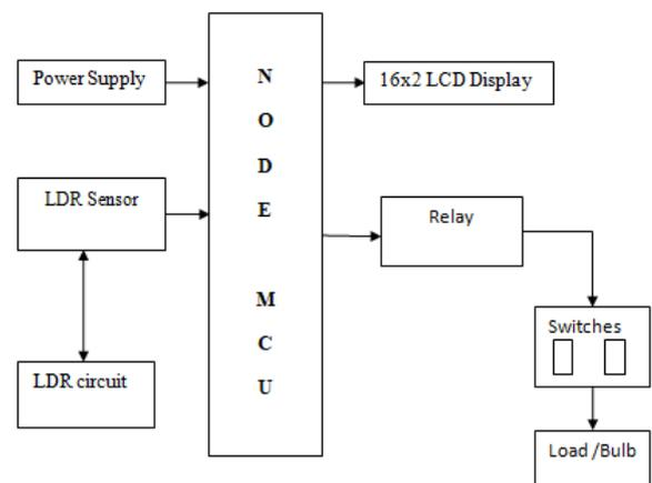
**Fig 3.Proposed Architecture for Smart Power**
