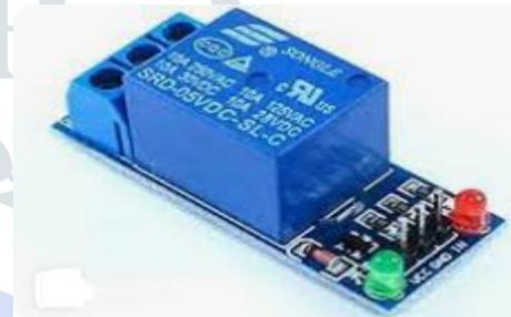
Fig.5: Relay Module
