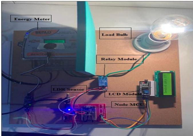
Fig.18: Designed hardware kit for Smart Power
