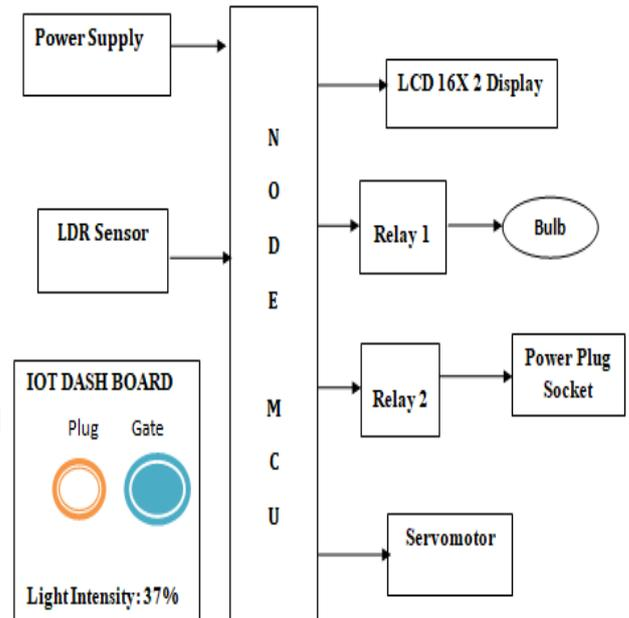
**Fig 2.Proposed Architecture for Smart Lighting, Smart Plug, Smart Gate System**
