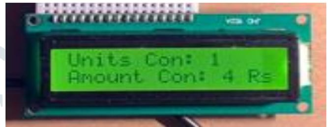
Fig.22: LCD shows that unit consumptions and cost of unit
