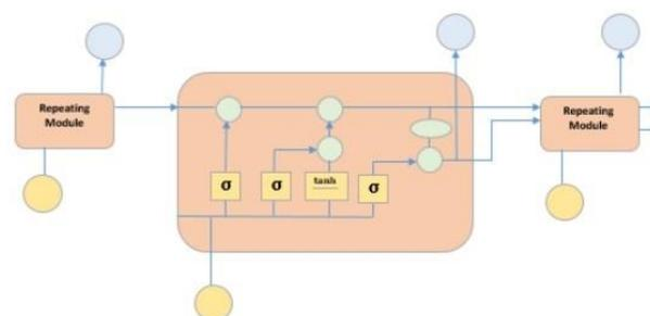
An LSTM module has a cell state and three gates which provide them with the power to selectively learn, unlearn or retain information from each of the units.
