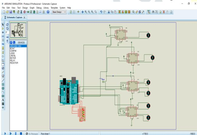
Fig.9 Driver based DC motor system
