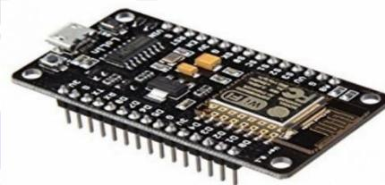
**Fig.6 NODEMCU with WIFI module**
