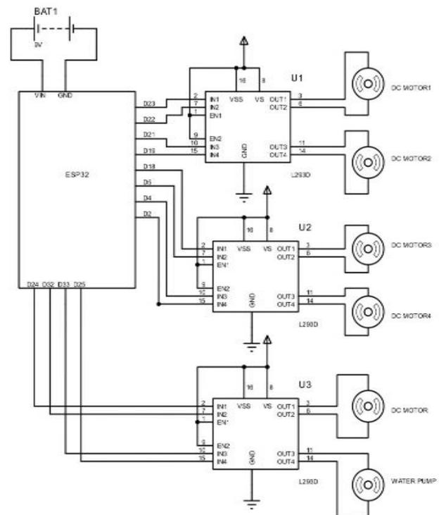
**Fig.2 Equivalent circuit of cleaning robot**
