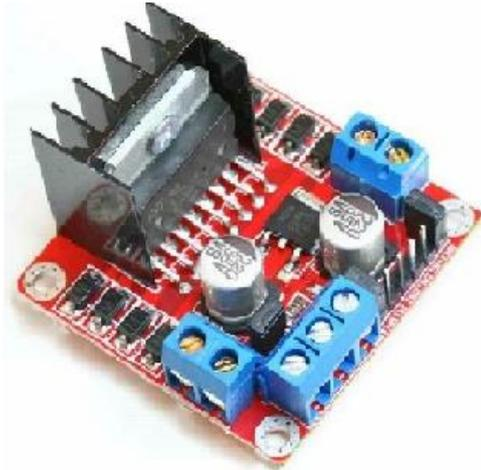
**Fig.3 Driver unit of robot**
