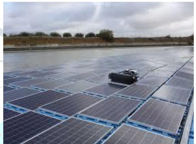
Fig.11 Snapshot of cleaning robot
