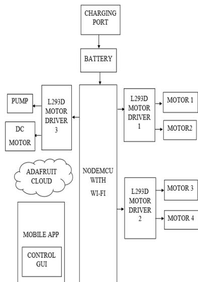
**Fig.1 Block diagram of cleaning robot**
