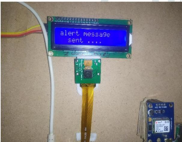
Using the GPS Module, a message alert is delivered to the user if they enter an invalid password, and it is displayed in the LCD here.
