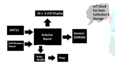
We are going to develop the weather monitoring system using the above illustrated blocks. The brain of the project is an Arduino board and the surrounding blocks are digital and analog sensors for acquiring local weather and environment data.
