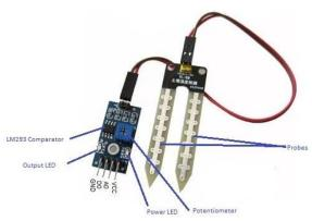
The soil Moisture sensor FC-28 has four pins
