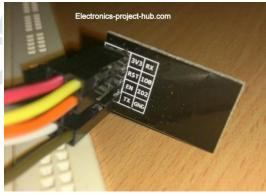
Pin Diagram of ESP8266
