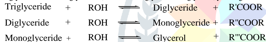
Scheme 3: The transesterification reactions of vegetable oil with alcohol to esters and glycerol
