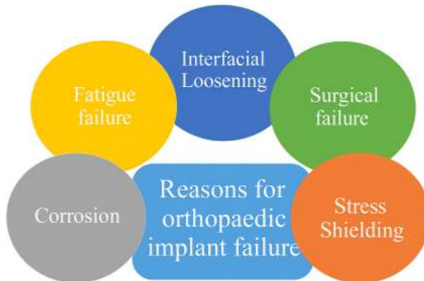
Figure 1 The factors responsible for secondary surgery due to implant failure.
