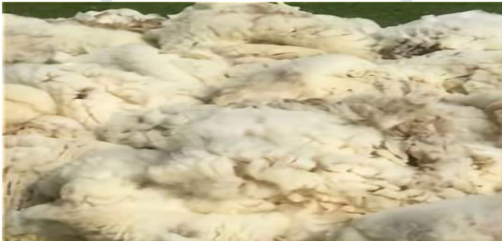
In place of chemical-laden insulation, sheep's wool is a great natural alternative. It insulates homes just as well as conventional insulation, but requires less energy to manufacture. One of the most eco-friendly ways to insulate your property, sheep's wool can both increase energy efficiency and soundproof your office.
