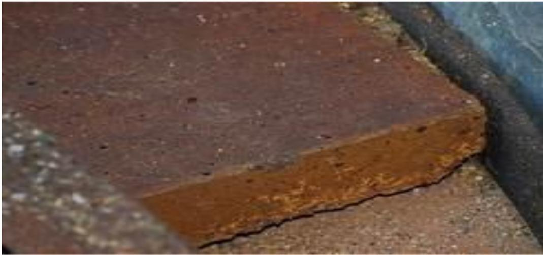
Another concrete alternative, ferrock is created with steel dust, or ferrous rock, left over from industrial processes, usually sent to the landfill. When combined with carbon dioxide, an iron carbonate is formed. This viable alternative to cement can be mixed and poured to form driveways, pathways, staircases and more
