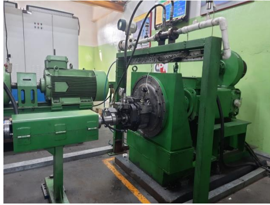
Fig.5- Testing of Gear Box
