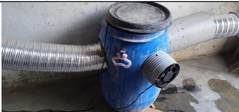
Alternatively, PVC pipe ducting can be used. A duct system allows the design of an indirect evaporative cooling system for homes with improper ventilation. The absence of windows and access to fresh external air can pose a design constraint. However, using PVC or Aluminium Chimney duct systems can be designed (Carsten 2020).
