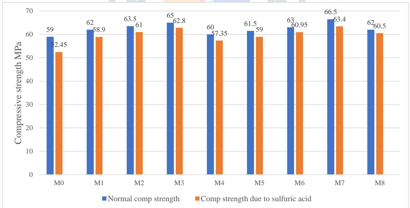
**Figure 7: compressive strength of cubes after performing an acid attack**
