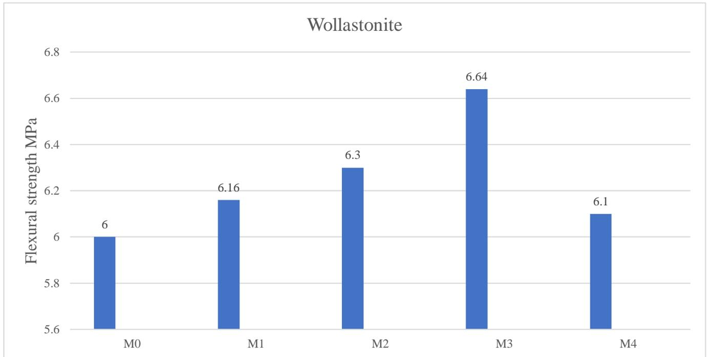
**Figure 5: Relation between % wollastonite replacement and flexural strength**
