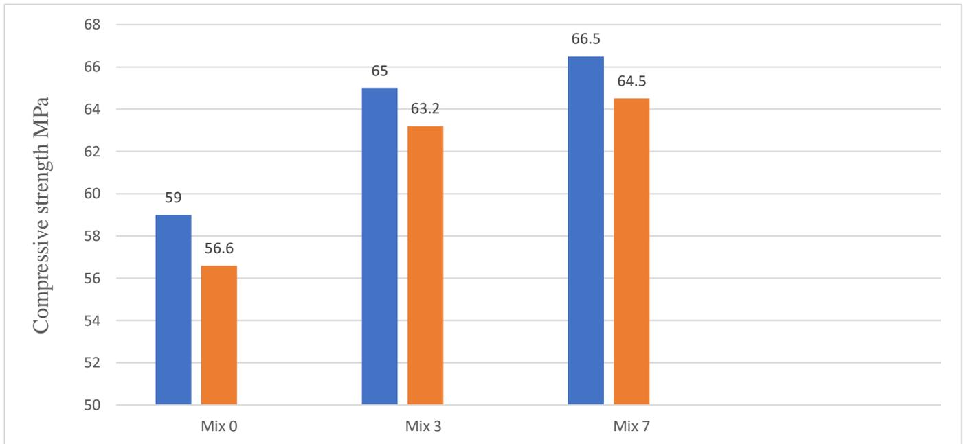
**Figure 9: compressive strength of cubes after Chloride attack**
