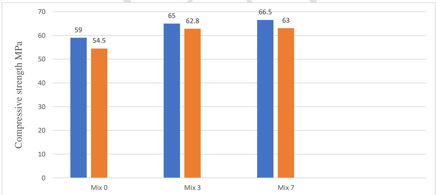
**Figure 8: compressive strength of cubes after sulphate attack**
