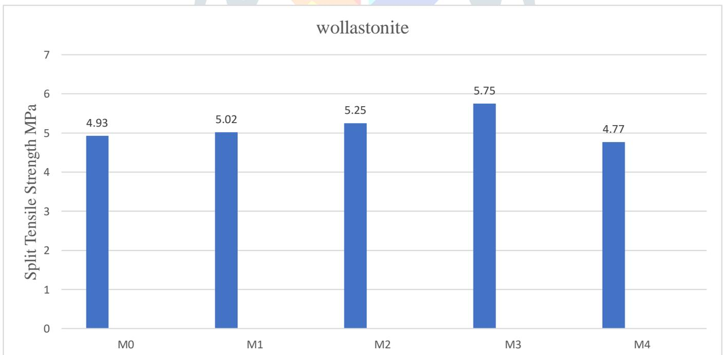
**Figure 3: Relation between % wollastonite replacement and split tensile strength**
