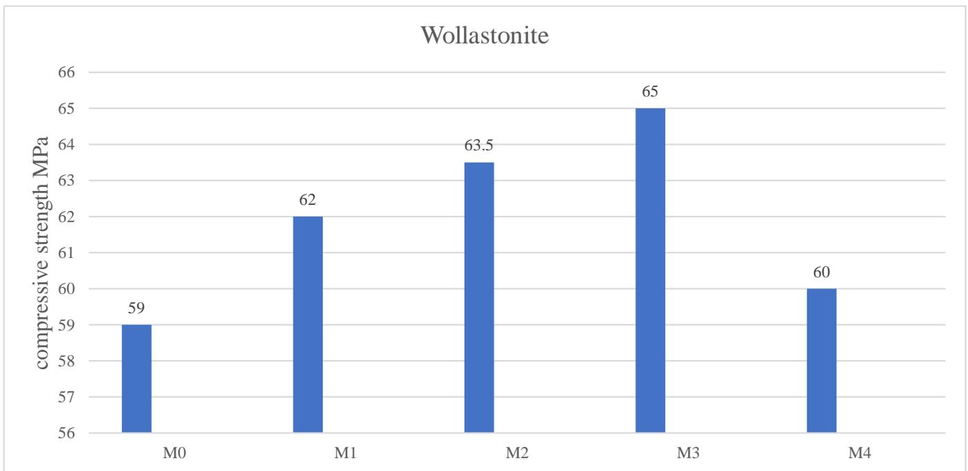
**Figure 1: Relation between % wollastonite replacement and compressive strength**
