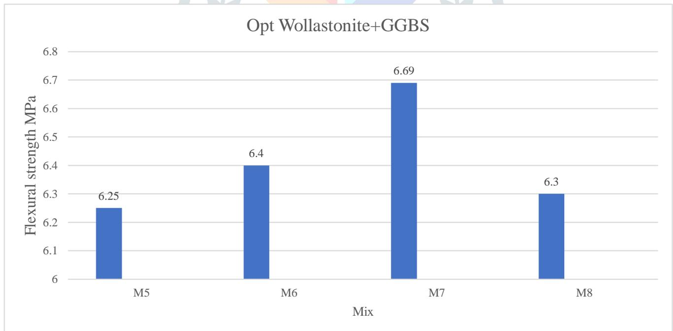
**Figure 6: Relation between opt wollastonite(15%)+%GGBS replacement and flexural strength**
