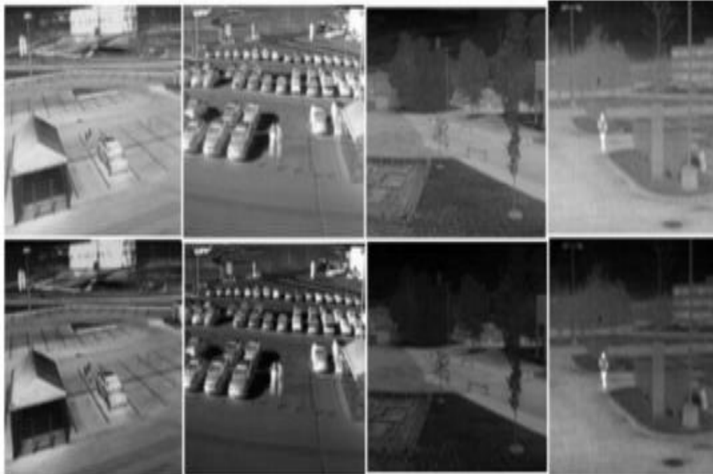
Fig. 5: Pre-processing of thermal images using Gamma correction
