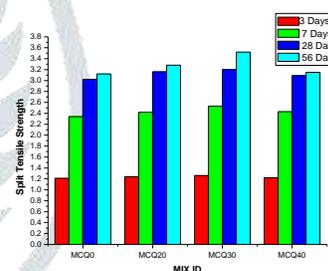
Fig.4 Differences in split tensile strength for various mix id C.FLEXURAL STRENGTH
