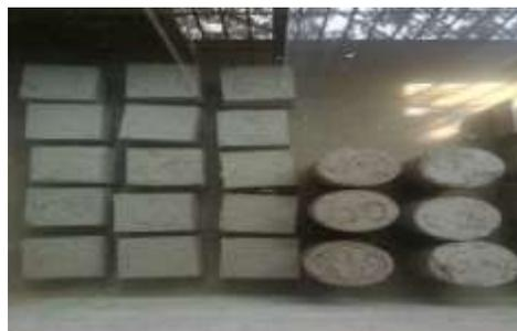
Figure 1. Samples placed in Curing pond for Curing
