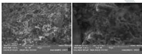
From the 2.5kx-, 5kx-, and 7.5kx-SEM images of normal concrete mix specimen, it is evident that a higher amount of fly ash is bound with the cement particles, while silica fumes appear as white collated balls. The composition of conventional concrete, prepared with fly ash and silica fume as admixtures, sheds light on the binding capability of cement and admixtures with other ingredients, as well as the density of the concrete.
