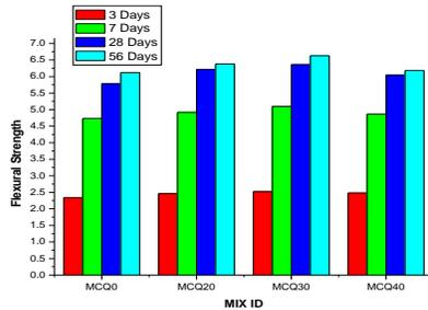
Fig.5 Fig.5 Differences in Flexural strength for various mix id
