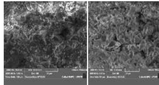
Fig.7 Scanning Electron Microscopic (SEM) Images of Modified Quartzite waste Concrete at 3kx and 2kx and 1.5kx Magnifications
