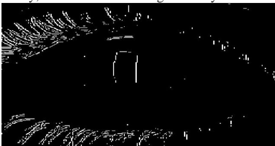
Fig3: Edge detection by Sobel filter
