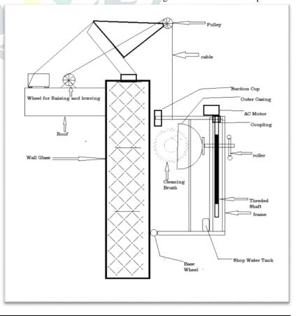
**OBJECTIVE:** Objective of this machine to clean glass window with motor operator brush.
