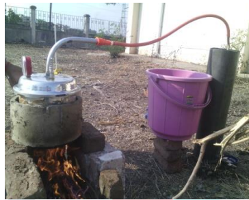
fig.9. Experimental setup for production of fuel from plastic waste.
