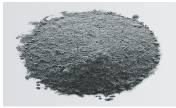
fig.8. Coal fly ash as catalyst
