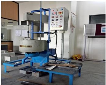
Fig. 3.1 Stir casting
