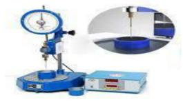
This test is performed to determine the consistency and hardness of bitumen material. The penetration value is determined as the vertical distance travelled by a standard needle to penetrate into bituminous material under specific condition of time, load and
