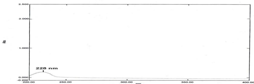
Fig:2 Maximum UV absorption of nizatidine hydrochloride at pH 1.2 is \lambda_{\max} 228 nm.
