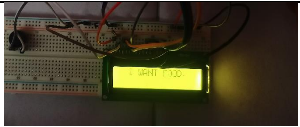
Fig 4: Displaying the message when the patient hand is in the direction of -x axis.
