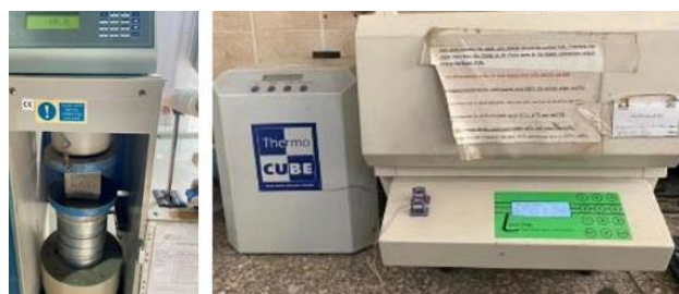
Figure 4 Used Measurement Instruments a) compressive strength machine b) laser comp heat flow meter fox
