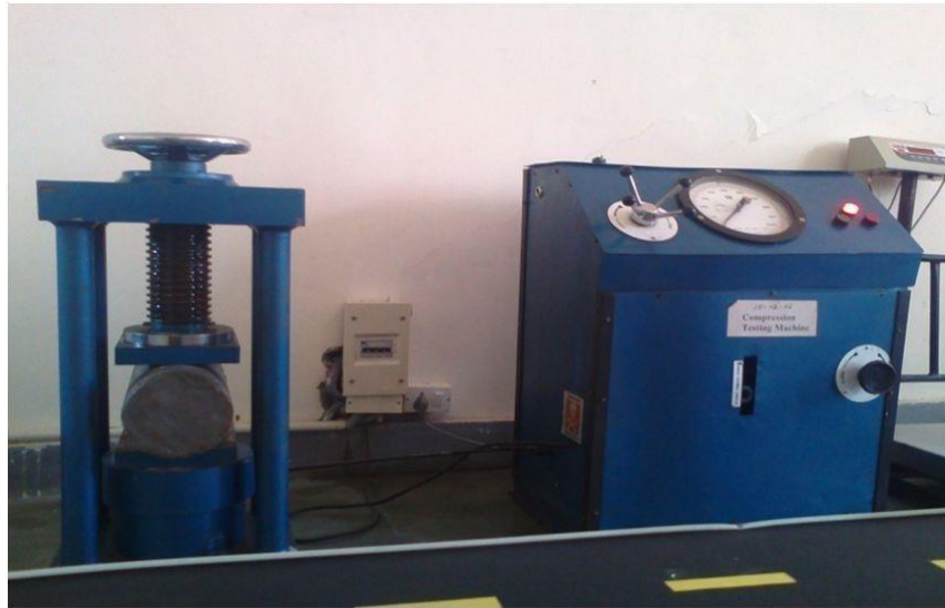
Fig. 9: Test Set up for Split Tensile Strength
