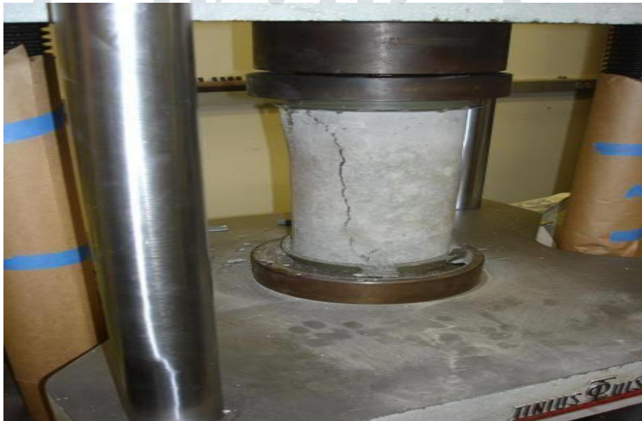
Fig. 8: Concrete specimen on Compressive Strength Testing Machine
