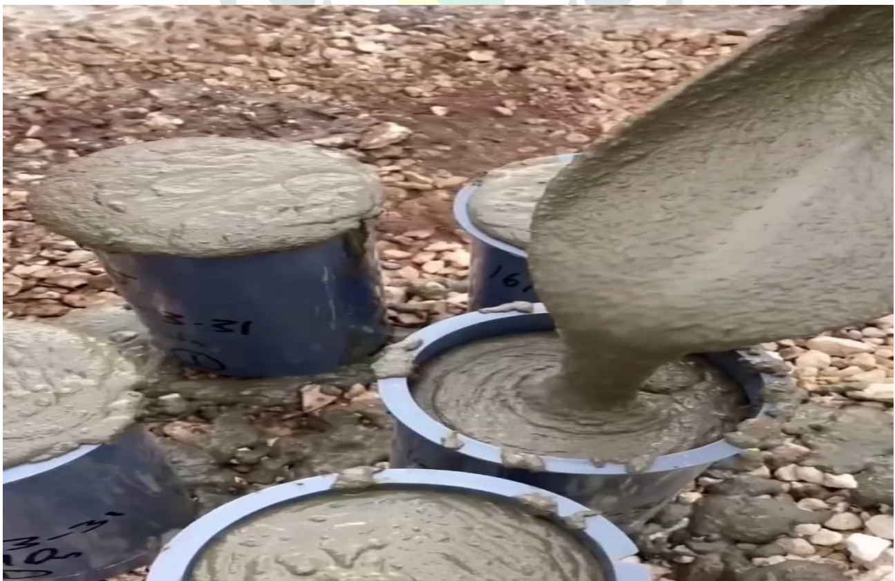
Fig. 7: Casting of Cylinder
