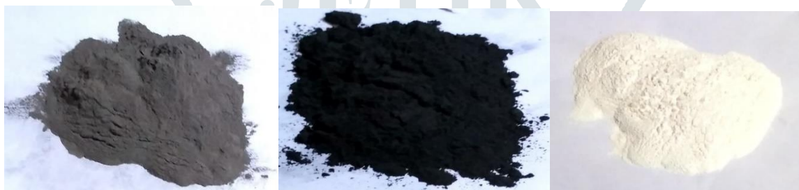
Fig.2.1 (a) Titanium carbide Powder, (b) Graphite powder, (c) Egg shell Powder
