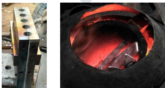
Fig. 2 (a) Mold used for casting, (b) Melting of Al7075
