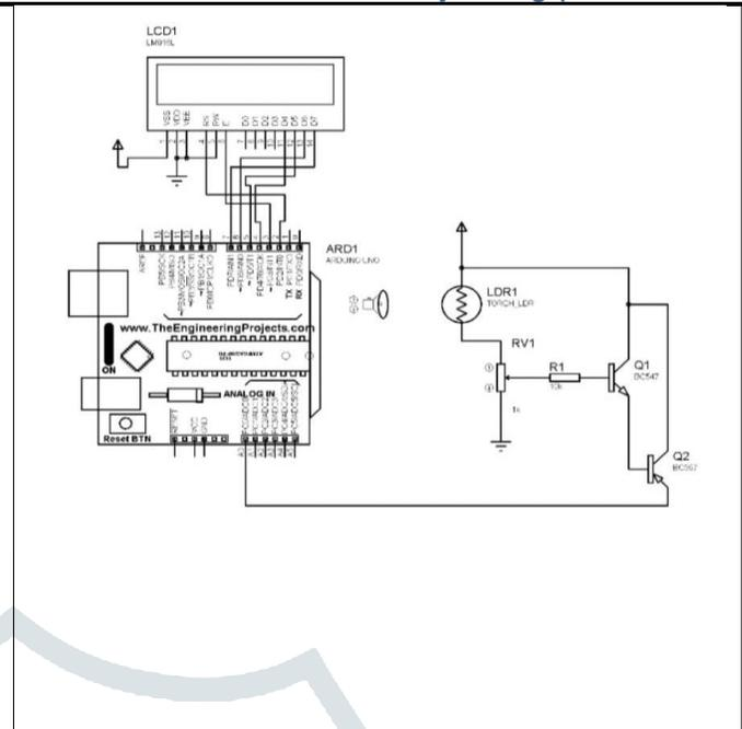
Fig. 2. Circuit diagram IV Drip Monitoring Device
