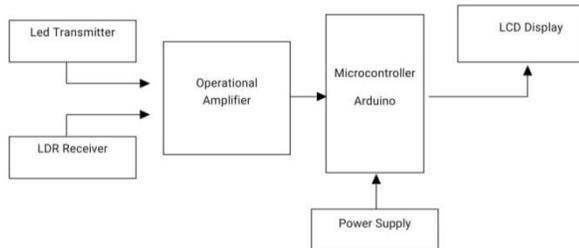
Fig. 1. Block Diagram of IV Drip Monitoring Device
