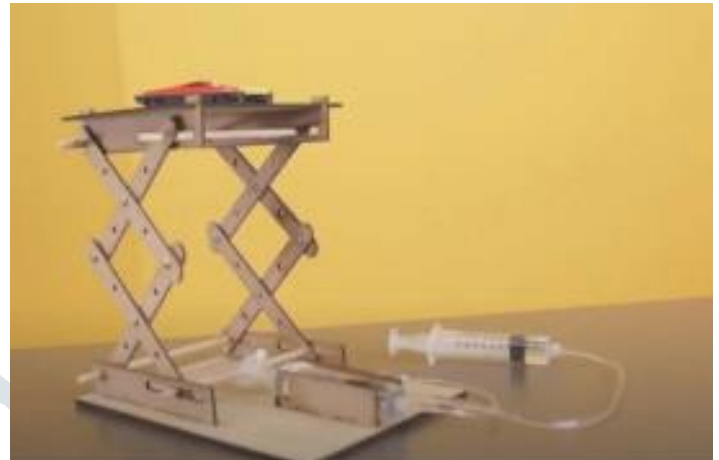
Fig -9: Prototype of hydraulic scissor lift
