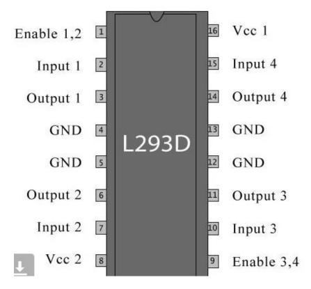
The L293D is a 16 pin IC, with eight pins, on each side, dedicated to the controlling of a motor. There are 2 INPUT pins, 2 OUTPUT pins and 1 ENABLE pin for each motor. L293D consist of two H-bridge. H-bridge is the simplest circuit for controlling a low current rated motor.
