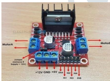
Fig.4: L298D Pin Diagram.[4]
