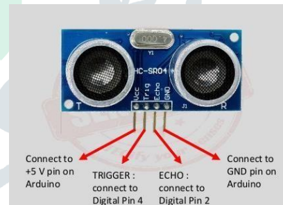
Fig.5: Ultrasonic Sensor HS-SR04. [5]
