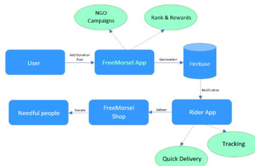
Fig 1.1 Basic flow of the application
