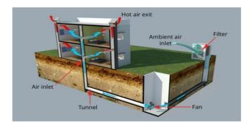
The cost of the compressor, condenser, and evaporator is eliminated by using this technique. merely utilizing geothermal power.
